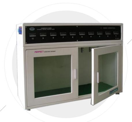
Purpose: Special used in testing glutinosity about the stickiness straps under normal temperature. The testing show that the stickiness straps pasted on the testing board under normal temperature can resist some displacement under gravity. The time of moving away some distance (or disengage completely) or move away (or disengage completely) within some time can show glutinosity about the stickiness straps.
